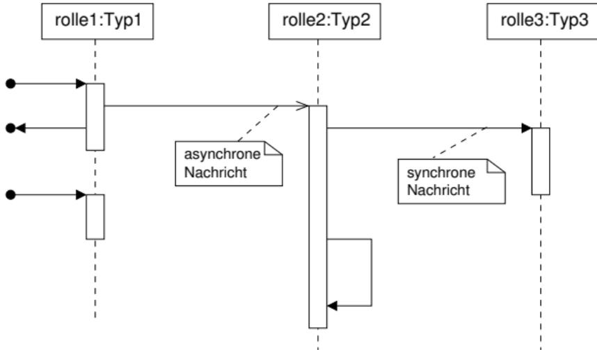
The sending object continues its processing after sending an asynchronous message (i.e., it works in parallel with the receiver).
