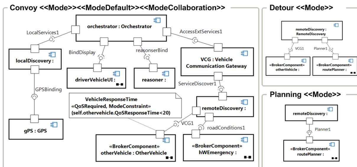
Figure 10: In-Vehicle service brokering architecture with Modes profile
