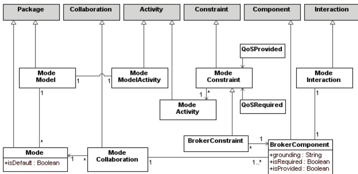
Figure 9: A Metamodel for service modes and service brokering specification (includes some highlighted UML classes)
