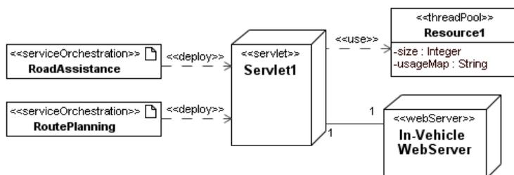
Figure 13: Example Deployment Model for two Service Orchestrations and one Servlet
