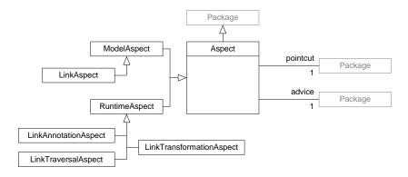
Fig. 2. Extension of UML metamodel
