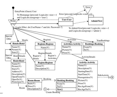
Figure 29. OO-H: navigation access diagram
