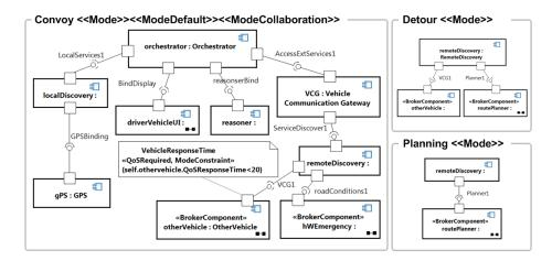
Fig. 10. Emergency service brokering architecture with Modes profile
