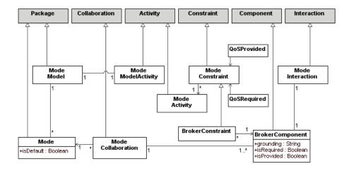
Fig. 9. Metamodel for service modes and service brokering specification (includes some highlighted UML classes)
