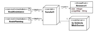
Fig. 13. Example: Deployment model for two service orchestrations and one servlet
