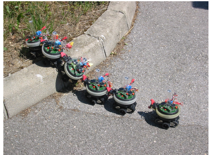
Figure 3. Robot swarm passing a step. Engineers must carefully evaluate how ensembles behave in the face of unforeseen difficulties such as overcoming an obstacle. (Photo courtesy of Francesco Mondada of the École Polytechnique Fédérale de Lausanne.)
