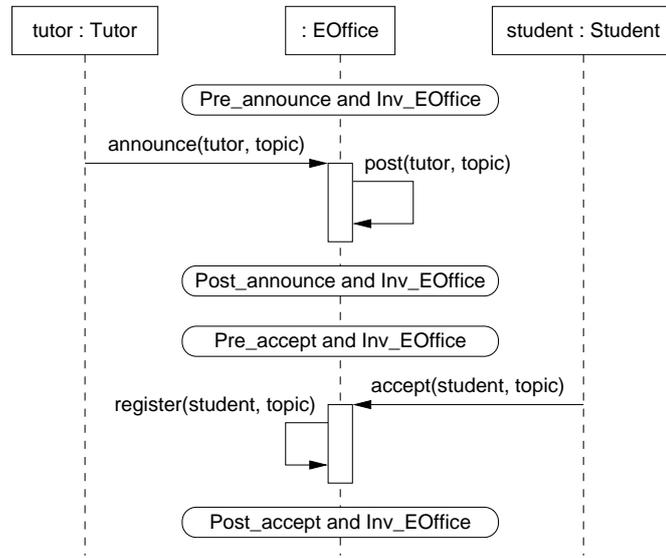
Fig. 7. E-office example: sequence diagram incl. OCL sentences for accepting a topic
