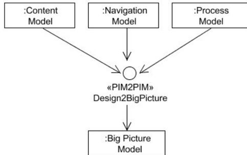
Figure 15: Transformations to build “big picture” model
