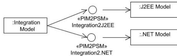
Figure 18: Generation of platform specific models
