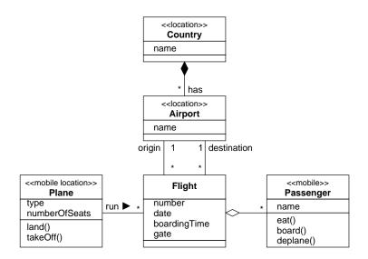
Fig. 2. A simplified class diagram modeling an airport.
