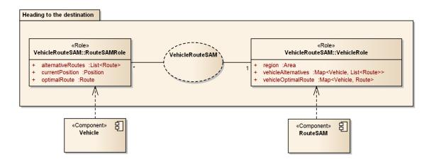
**Membership condition:** The ensemble should be formed whenever the vehicle's current position is within the managed area of the respective RouteSAM. Following DSL (Java) form it could be defined in the following way:
