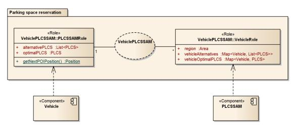
**Membership condition:** The ensemble should be formed whenever the vehicle's immediate destination is within the area that is managed by the PLCSSAM. Formally, it could be written as:
