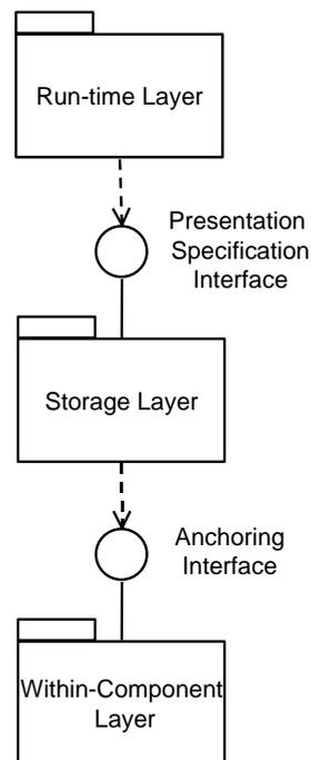
Figure 2: UML-Model for the Layers of the Dexter Hypertext Reference Model
