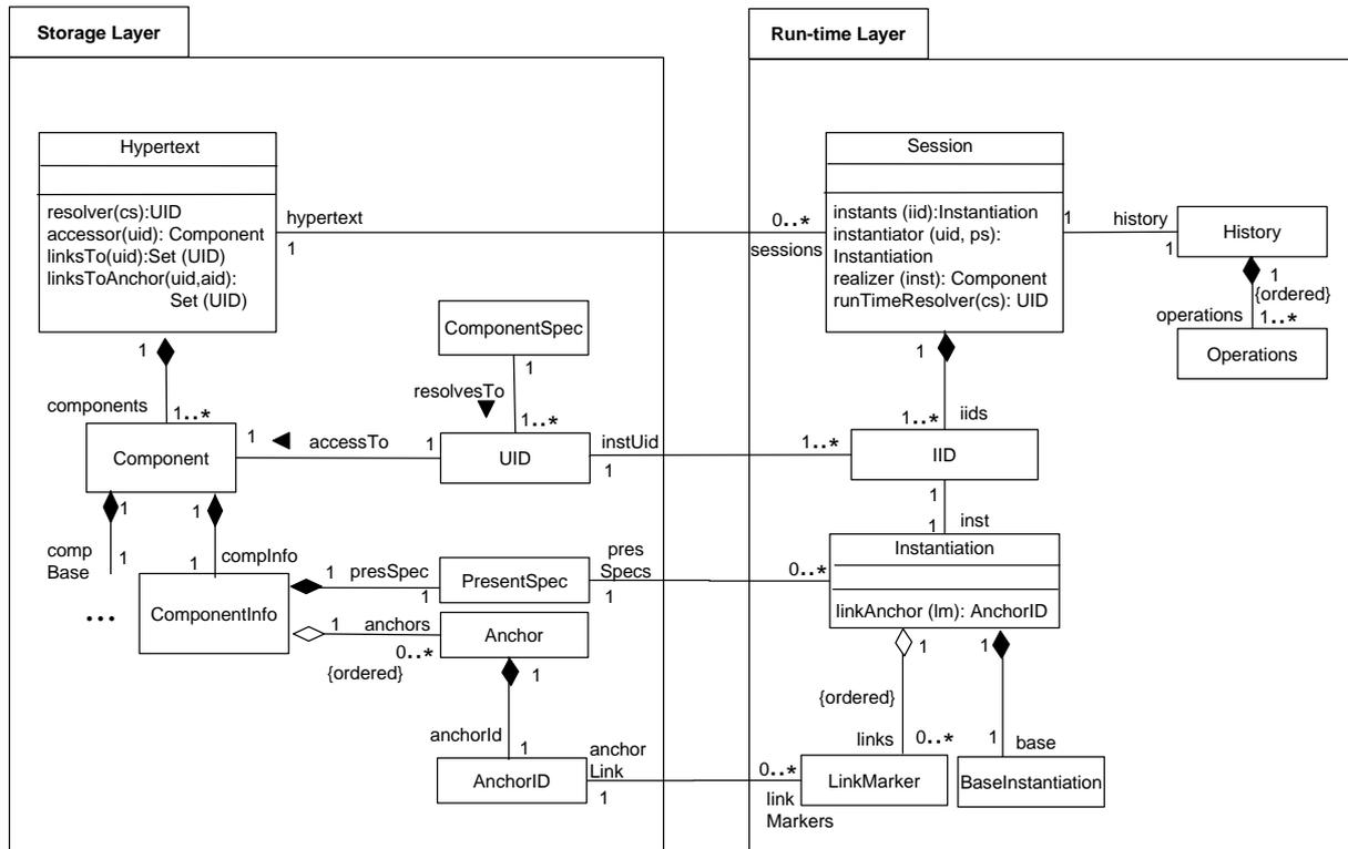
Figure 5: UML Class Diagram for the Run-time Layer and Part of the Storage Layer
