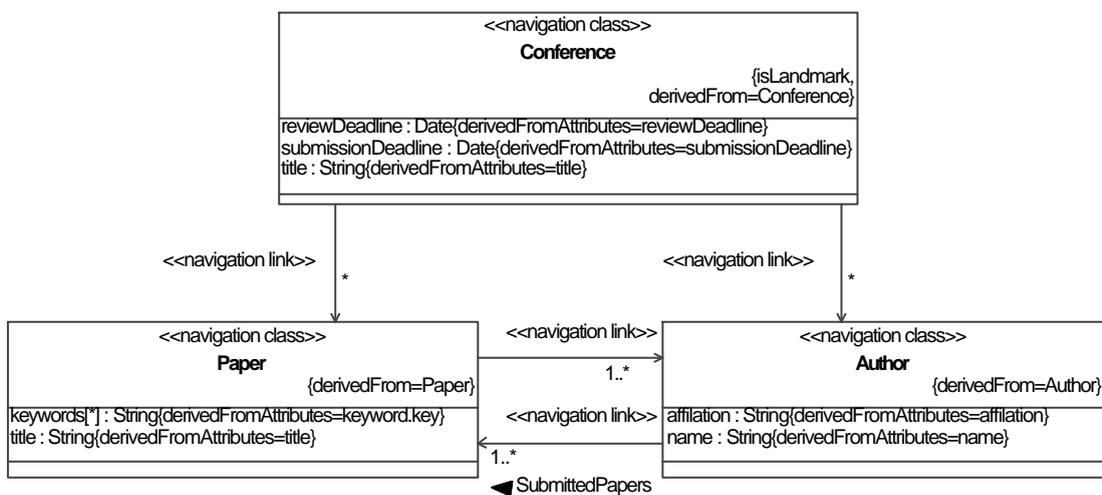
Figure 14. Example for a navigation model using the UWE UML profile
