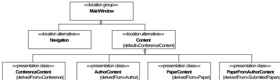
**Figure 15. Example for a presentation model using the UWE UML profile**
