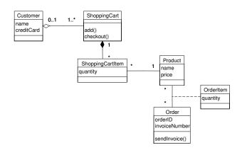
Fig. 3. Conceptual model of the e-shop example.
