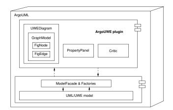
Fig. 7. Overview of the ArgoUWE plugin architecture.
