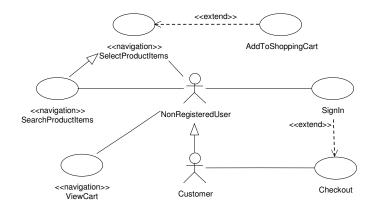
Fig. 2. Use case model of the e-shop example.
