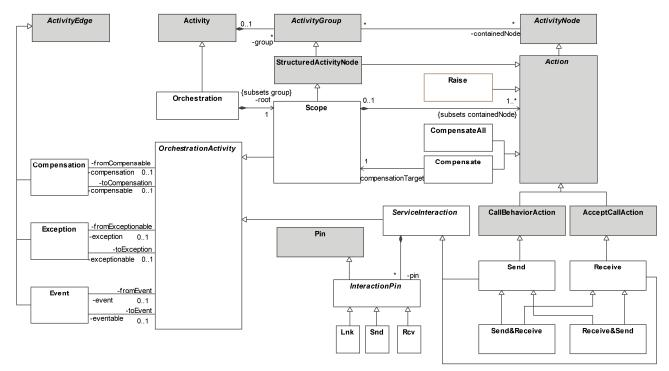
Figure 2: UML4SOA Metamodel (UML metaclasses in grey)
