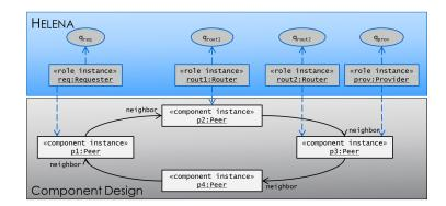
Fig. 5: A state of an ensemble in the p2p example with four role instances and four component instances where the peer p4 does not adopt any role, but the peer p3 adopts two roles in parallel.
