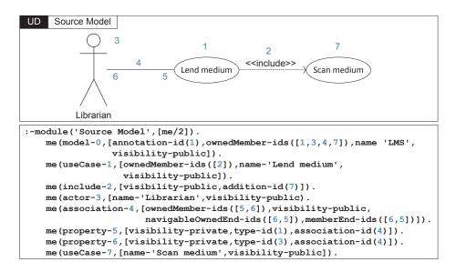
Fig. 1. A use case diagram (top) and its encoding as a Prolog fact database (bottom)
